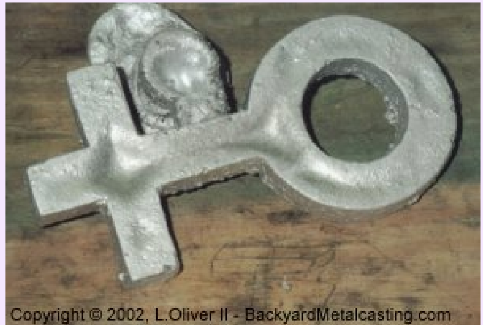
Figure 11.22 Some common defects in castings: (d) shrinkage cavity
