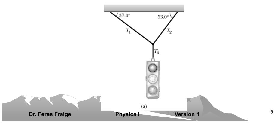
A traffic light weighing 122 N hangs from a cable tied to two other cables fastened to a support, as in Figure 5.10a. The upper cables make angles of 37.0° and 53.0° with the horizontal. These upper cables are not as strong as the vertical cable, and will break if the tension in them exceeds 100 N. Will the traffic light remain hanging in this situation, or will one of the cables break?
