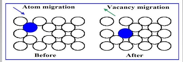
To jump from lattice site to lattice site, atoms need energy to break bonds with neighbors, and to cause the necessary lattice distortions during jump. This energy comes from the thermal energy of atomic vibrations ( $E_{\rm av} \sim kT$ )
