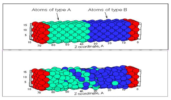
Inhomogeneous materials can become homogeneous by diffusion. For an active diffusion to occur, the temperature should be high enough to overcome energy barriers to atomic motion.
