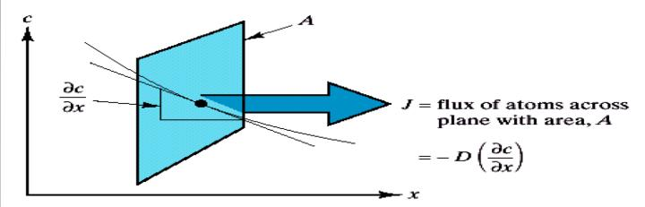
The concentration gradient is often called the *driving force* in diffusion (but it is not a force in the mechanistic sense).
