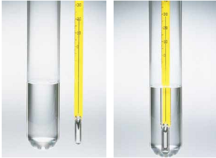
Figure 19.2 As a result of thermal expansion, the level of the mercury in the thermometer rises as the mercury is heated by water in the test tube.
