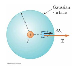
A spherical Gaussian surface of radius r surrounding a point charge q. When the charge is at the center of the sphere, the electric field is everywhere normal to the surface and constant in magnitude.
