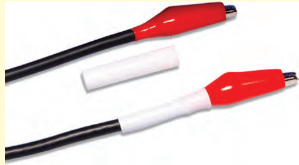
Photograph showing (from top to bottom) an electrical connection, a piece of as-received polymer shrink-tubing, and the constricted tubing around the junction—application of heat to the tubing caused its diameter to shrink. (Photography by S. Tanner.)
