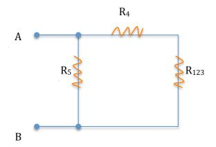
$R_{123}$  and  $R_4$  are connected in Series, Thus  $R_{1234}$  is  $R_{1234}\!=\!R_{123}+R_4\!=\!5\!+\!20\!=\!25\Omega$
