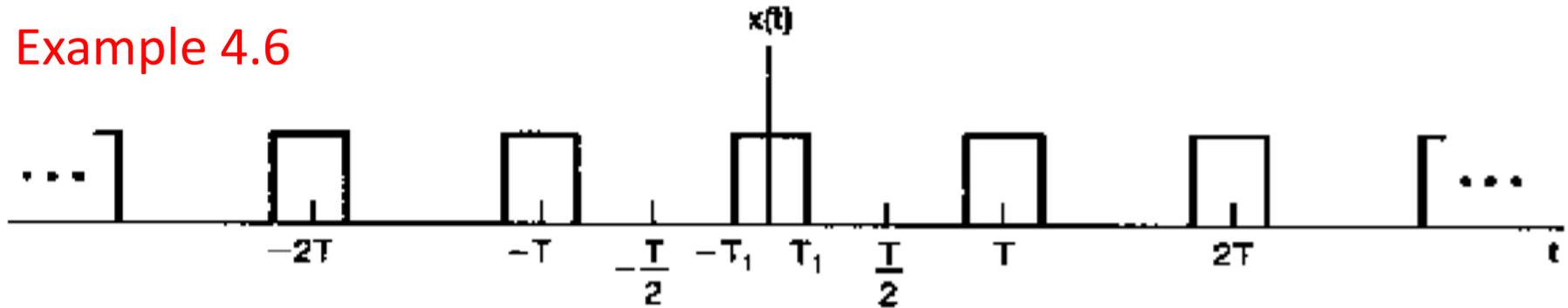
The Fourier series coefficients of the above periodic signal:  $a_k = \frac{\sin(k\omega_0 T_1)}{\pi k}$
