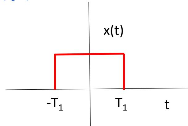
$$\begin{aligned} X(j\omega) &= \int_{-T_1}^{T_1} 1 \cdot e^{-j\omega t} dt = \frac{e^{-j\omega t}}{-j\omega} \Big|_{-T_1}^{T_1} = -\frac{1}{j\omega} \left[ e^{-j\omega T_1} - e^{j\omega T_1} \right] \\ &= \frac{1}{j\omega} \left[ e^{j\omega T_1} - e^{-j\omega T_1} \right] = \frac{2j \sin(\omega T_1)}{j\omega} = \frac{2 \sin(\omega T_1)}{\omega} \end{aligned}$$
