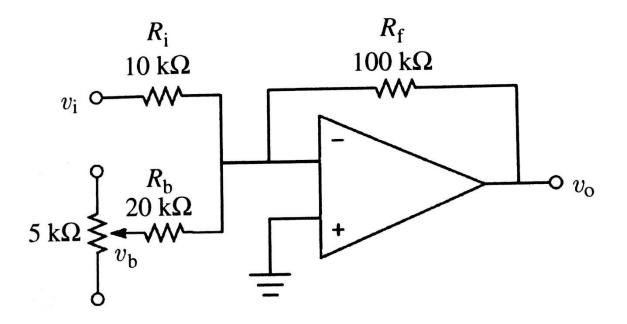
The undesired voltage at  $v_i$ = 5 V. For  $v_o$ = 0 V, the current flowing through R<sub>f</sub> should be zero.
