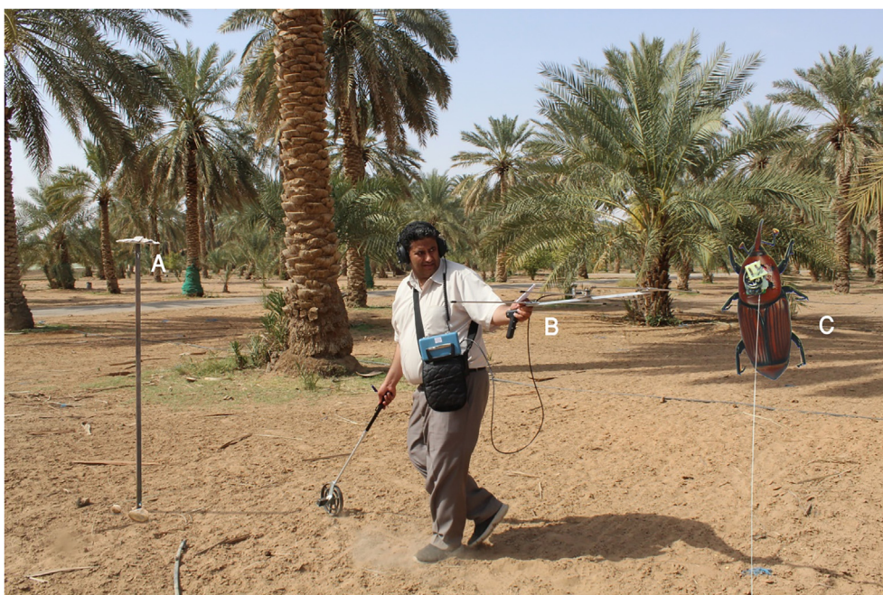
Fig. 3. Date palm orchard showing release point (platform A), receiver TRX 2000S (B), and tagged adult (C).
