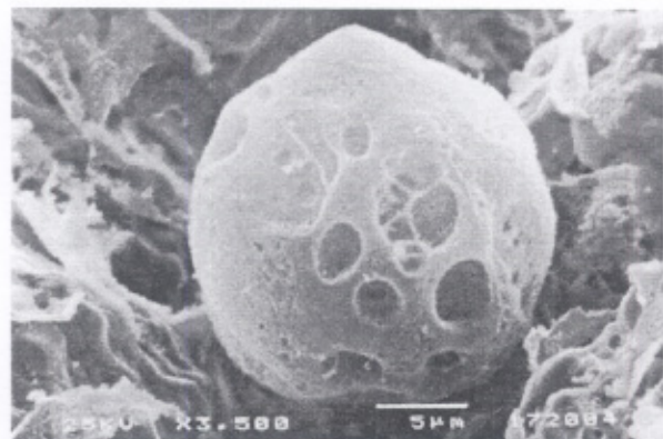
Fig 3. Scanning electron micrograph of PDL fibroblasts incubated with amalgam for 72 hours. The cell is round in shape with different sizes of vacuoles (original magnification \times 3500 ).
