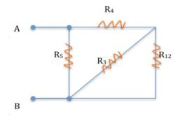
R<sub>1</sub> and R<sub>2</sub> are connected in Series, Thus R<sub>12</sub> is R<sub>12</sub>=R<sub>1</sub> + R<sub>2</sub> = 10Ω since R<sub>12</sub> and R<sub>3</sub> are connected in Parallel, Thus R<sub>123</sub> is  $\frac{1}{R_{123}} = \frac{1}{R_{12}} + \frac{1}{R_3} \Rightarrow \frac{1}{R_{123}} = \frac{1}{10} + \frac{1}{10}$ R<sub>123</sub> = 5Ω R<sub>4</sub> A R<sub>5</sub> B
