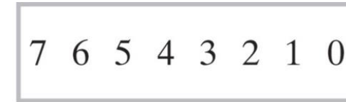
(b) Individual bits of 8-bit register
