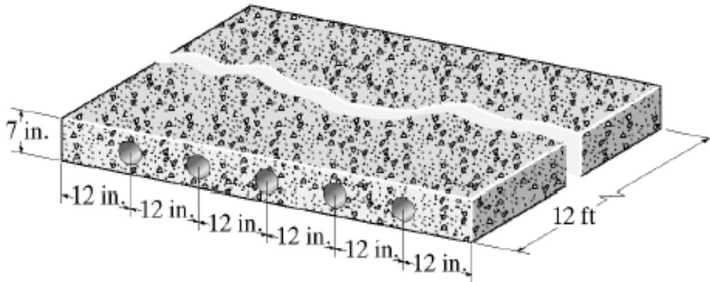
$$W = (144 \text{ lb/ft}^3)[(12 \text{ ft})(6 \text{ ft})(\frac{7}{12} \text{ ft}) - 5(12 \text{ ft})(\pi)(\frac{2}{12} \text{ ft})^2] = 5.29 \text{ k} \quad \text{Ans}$$
