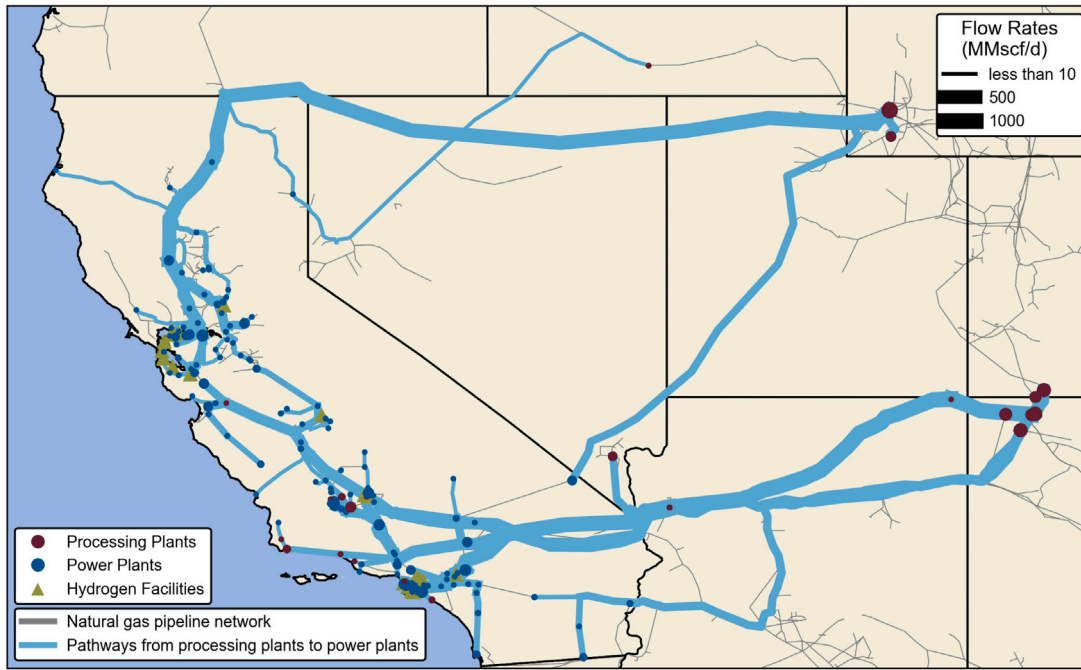
Fig. 2. Natural gas supply pathways to California power plants. The map illustrates the natural gas supply chain for California power generation sector: light blue lines represent simulated supply pathways from processing plants to power plants. Line thickness corresponds to the volumetric flow rate (MMscf/d), and node size reflects the facility’s capacity. Green triangles denote the hydrogen facilities which are distributed in Bay Area, Los Angeles, and Bakersfield. (For interpretation of the references to color in this figure legend, the reader is referred to the web version of this article.)
