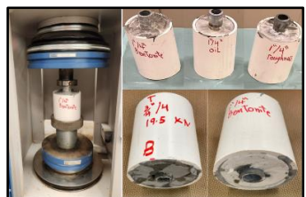
Fig. Error! No text of specified style in document. Cement-Casing Bond Strength Testing
