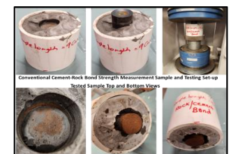
Fig. 9 Conventional C/C Bond Strength Testing
