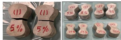
Fig. Error! No text of specified style in document. Direct (Pull) Tensile Strength Testing
