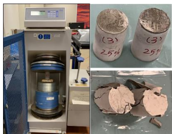
Fig. Error! No text of specified style in document. Uniaxial Compressive Strength Testing
