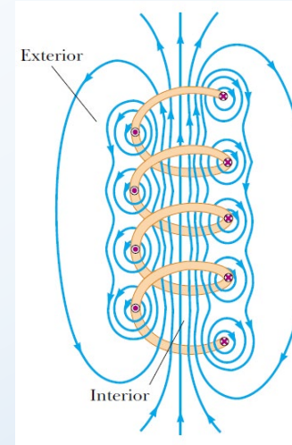
The magnetic field lines for a loosely wound solenoid.
