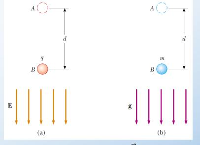
(a) When the electric field  $\vec{E}$  is directed downward, point *B* is at a lower electric potential than point *A*. When a positive test charge moves from point *A* to point *B*, the charge-field system loses electric potential energy. (b) When an object of mass *m* moves downward in the direction of the gravitational field *g*, the object-field system loses gravitational potential energy.
