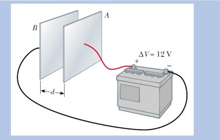
A 12 V battery connected to two parallel plates. The electric field between the plates has a magnitude given by the potential difference  $\Delta V$  divided by the plate separation *d*.
