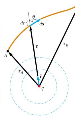
The potential difference between points A and B due to a point charge q depends <u>only</u> on the initial and final radial coordinates  $r_A$  and  $r_B$ . The two dashed circles represent intersections of spherical equipotential surfaces with the page.
