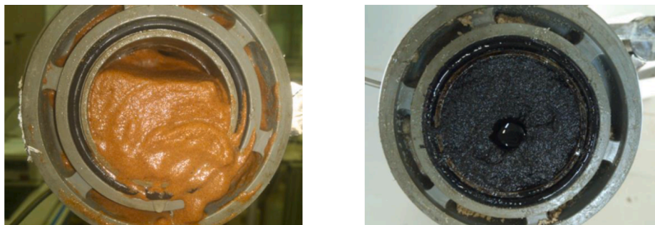
Fig. 9. Outlet end erosion profiles at the end of water and crude oil displacement without filter.
