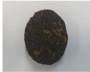
Fig. 11. Filter condition after displacement of sand pack A with 90 cp crude oil.
