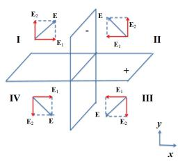
The total electric field is the resultant of the field  $\mathbf{E}_1$  due to the positively charged sheet and of the field  $\mathbf{E}_2$  of the negatively charged sheet. Both of them are everywhere perpendicular to each other and have the same magnitude  $\sigma/2\epsilon_0$ . Thus for the total field we have:
