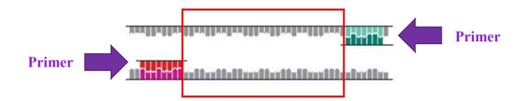
• From this information <u>two synthetic oligonucleotide primers</u> may be chemically synthesised each complementary to a stretch of DNA to the 3' side of the target DNA, one oligonucleotide for each of the two DNA strands (DNA polymerase can add a nucleotide only onto a **preexisting 3'-OH group**).
