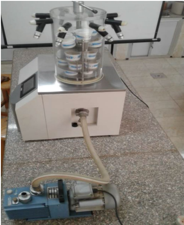
Fig. 1 Laboratory lyophilizer equipment (model: VaCo 5-D, S/N: COM98754, Zirbus Technology, Germany)
