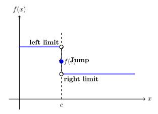
The function has a jump at x = c. Both one-sided limits exist but are not equal.
