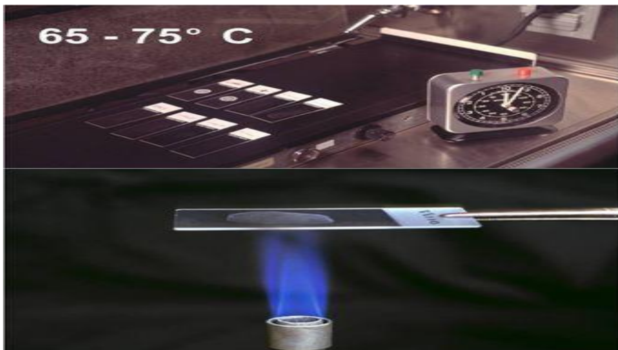
Heat Fixation of smear (Upper: using electric heater, lower: using burner)
