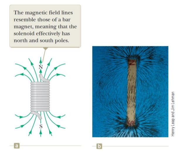
The magnetic field pattern of a bar magnet is displayed with small iron filings on a sheet of paper.
