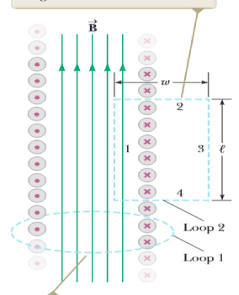
Ampère's law applied to the circular path whose plane is perpendicular to the page can be used to show that there is a weak field outside the solenoid. Because the solenoid is ideal, B in the interior space is uniform and parallel to the axis, and B in the exterior space is zero.
