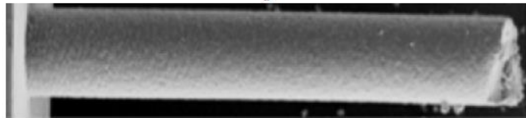
Image of a plastic footprint of a nozzle hole made with: a- laser; b- laser-EDM after drilling EDM.
