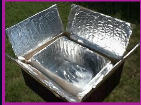
4 Flat Reflectors Open Corners
