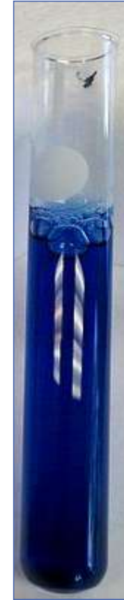
Test tubes containing: Bradford reagent with protein added. \lambda_{\max} is shifted to 595nm.
