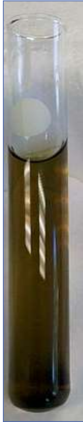
Test tube containing: Bradford reagent alone. \lambda_{\max} of the dye 465nm
