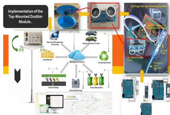
Fig. 11. Implementation of the Top-Mounted Dustbin Module.
