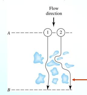
As solute molecules travel through the column, some arrive at the end sooner then others simply due to the different path traveled around the support particles in the column that result in different travel distances.
