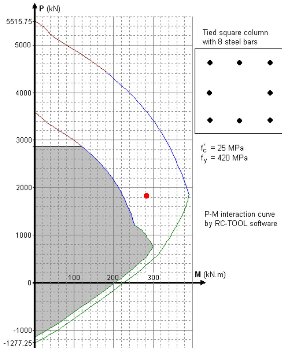
This point (1800, 283.5) is located in unsafe zone ... OK the column is not safe
