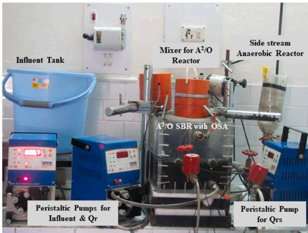
Fig. 2. (a) Schematic diagram of SBR with inlet anaerobic reactor, pre-anoxic chamber and side stream anaerobic reactors and (b) Picture of experimental set up.
