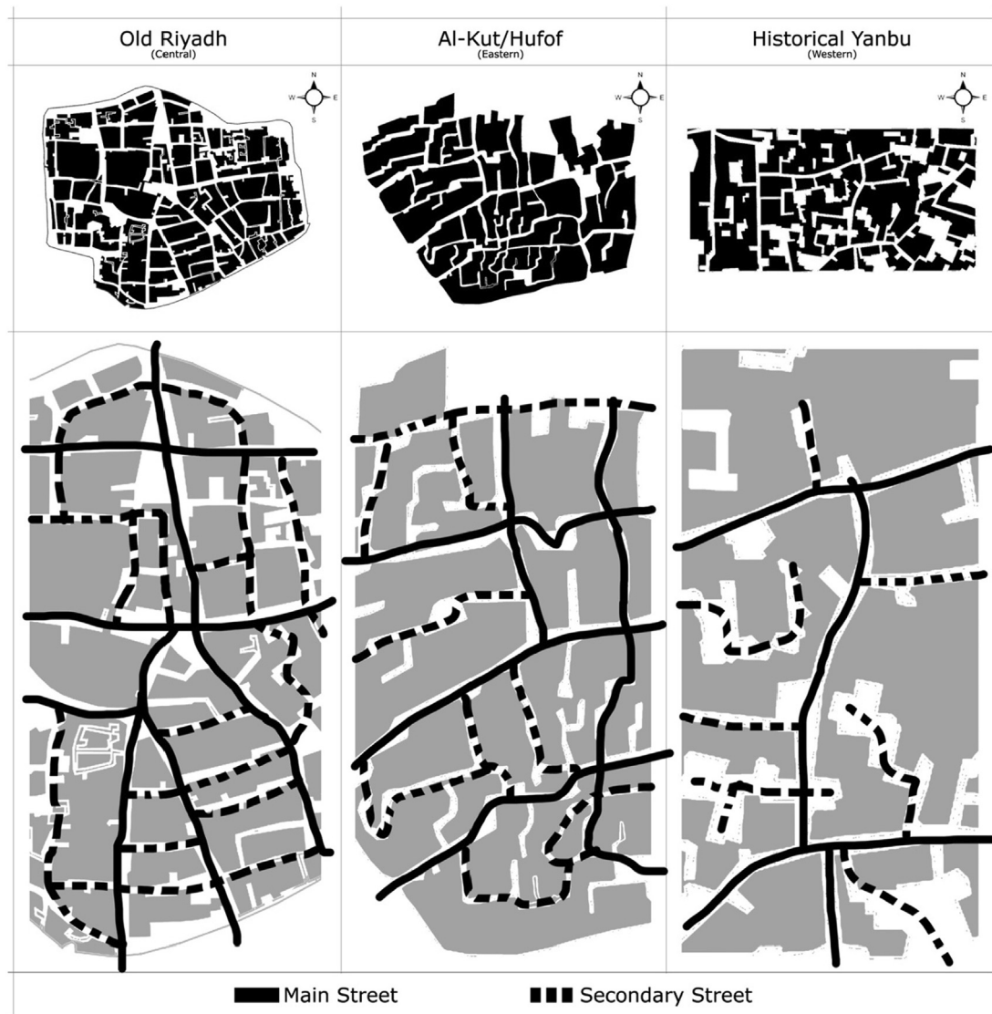
Fig. 12. Main streets interconnect to ensure the accessibility of public domain and preserve the privacy of private domain.
