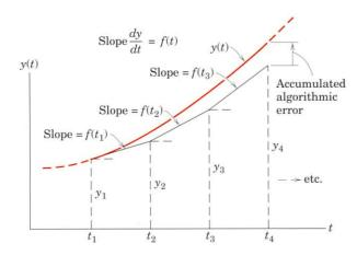
Beginning at  $t_1$ , at which the value  $y_1$  is known, we project the slope over a horizontal subinterval or step  $(t_2 - t_1)$  and see that  $y_2 = y_1 + f(t_1)(t_2 - t_1)$ . At  $t_2$ , the process may be repeated beginning at  $y_2$ , and so forth until the desired value of t is reached. Hence, the general expression is
