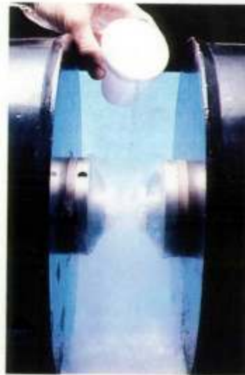
Figure 11.21 The paramagnetic properties of O_2 . Liquid O_2 is attracted to the poles of a magnet because it is paramagnetic, as MO theory predicts. A diamagnetic substance would fall between the poles.
