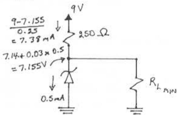
$$\begin{aligned}R_{L_{\min}} &= \frac{7.155}{7.38 - 0.5} \\ &= \underline{\underline{1.04 \text{ k} \Omega}}\end{aligned}$$
