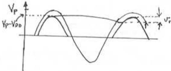
$$(i) \bar{V}_r \approx (V_p - V_{DD}) \frac{T}{CR} \quad \text{Eq. (3.28)}$$
