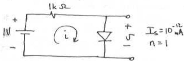
$$\#1 \quad V = 0.7 \text{ V} \quad i = \frac{1 - 0.7}{1} = 0.3 \text{ mA}$$
