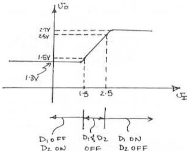
For  $U_I \geq 2.5V \sim D_1 \text{ on}$
