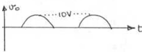
$$V_{p+} = \underline{10V} \quad V_{p-} = \underline{0V} \quad f = 1\text{kHz}$$
