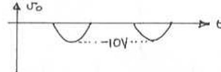
$$V_{p+} = \underline{0V} \quad V_{p-} = \underline{-10V} \quad f = 1\text{kHz}$$
