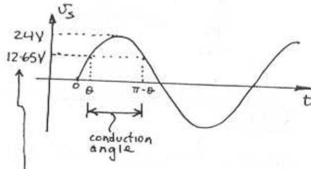
Conduction starts when  $V_s > 12 + V_{DD}$
