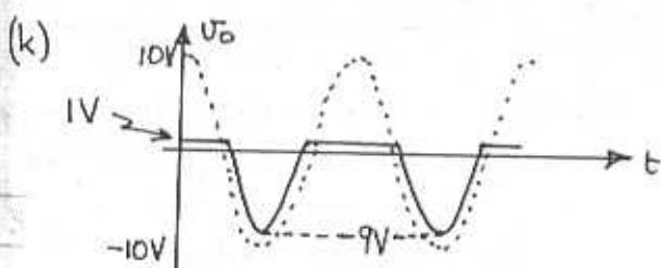
$$V_{p+} = \underline{1V} \quad V_{p-} = \underline{-9V} \quad f = 1kHz$$
