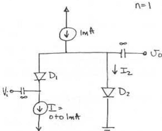
small signal model when  $D_1$  &  $D_2$  are conducting
