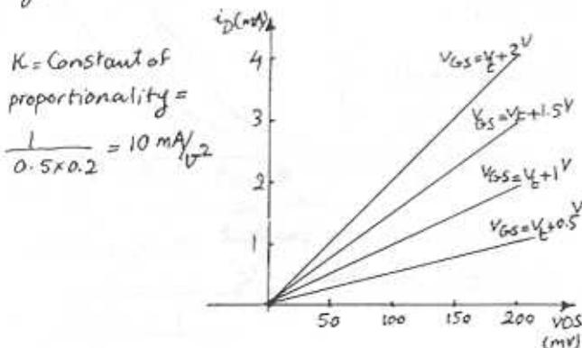
$$r_{DS} = \frac{i_D}{V_{DS}} = \frac{1}{0.2} = 5 \text{ k}\Omega \text{ for } V_{DS} = 0.5 \text{ V}$$
