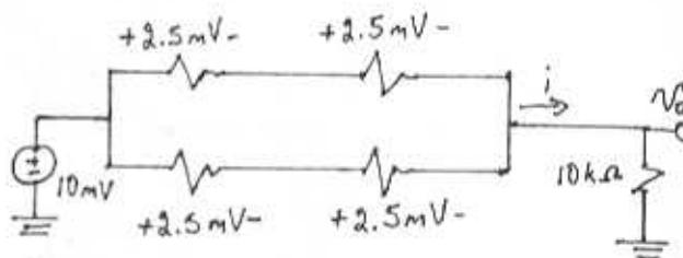
WE SEE THAT  $V_o = 5 \text{ mV}$  AND  $i = \frac{5 \text{ mV}}{10 \text{ k}\Omega} = 0.5 \mu\text{A}$ .
