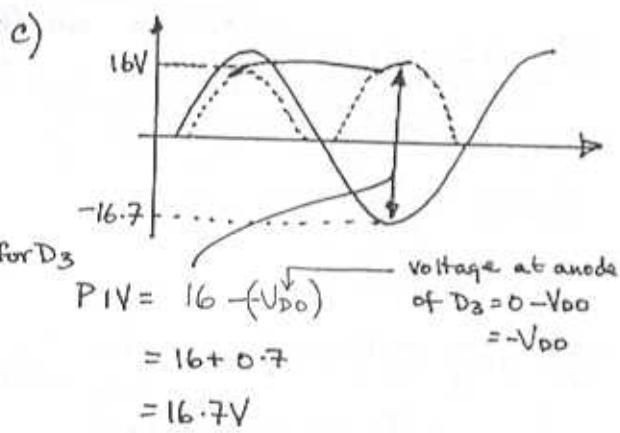
$$\text{Allowing a } 50\% \text{ margin} = 16.7 \times 1.5$$
