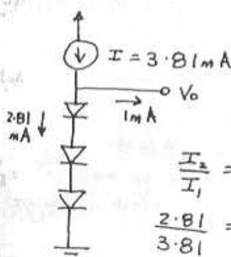
$$\frac{I_2}{I_1} = e^{\frac{(V_2 - V_1)/3}{0.025}}$$
