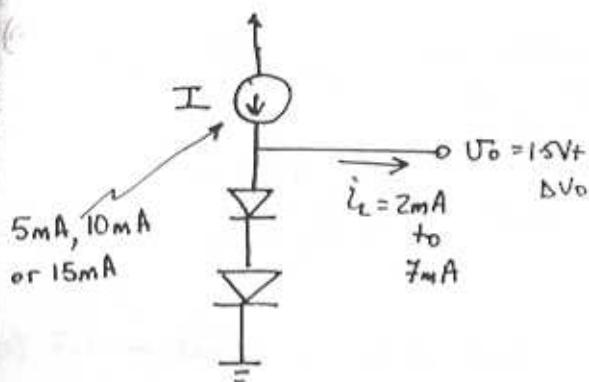
For a load current of 2 to 7 mA, I must be greater than 7 mA. Thus the 5 mA source would not do.
