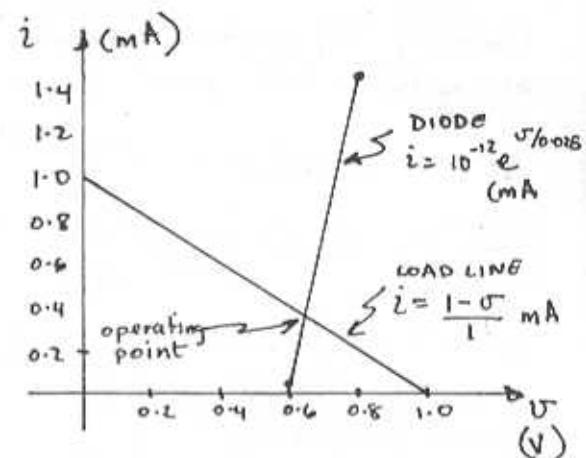
From the above sketch we see that the operating point must lie between  $V = 0.6$  and  $0.7 \text{ V}$  and  $i \times 0.3$  to  $0.4 \text{ mA}$ . To find the point more accurately an enlarged graph is plotted.
