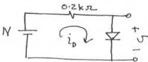
$$(a) \quad i_D = \frac{1 - 0.7}{0.2} = \underline{1.5 \text{ mA}}$$
