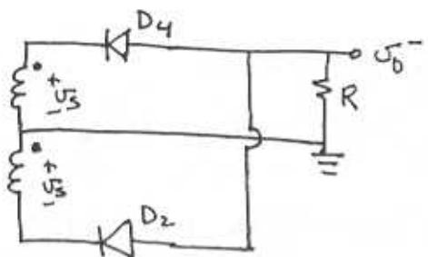
If choosing a diode, allow a safety margin of  $1.5 \text{ PIV} = \underline{\underline{73V}}$
