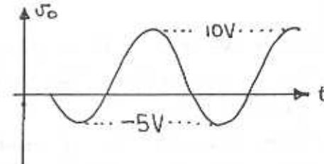
$$V_{p+} = \underline{10V} \quad V_{p-} = \underline{-5V} \quad f = 1\text{kHz}$$
