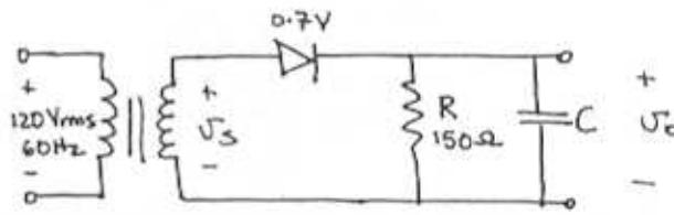
$$V_{O,\text{peak}} = V_p - V_{DD} = 16$$
