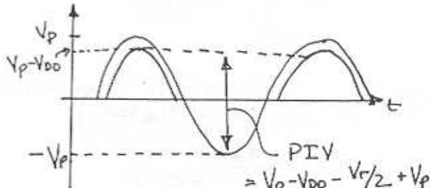
For a 50% safety margin  $\text{PIV} = 1.5 \times 31.7 \\ = \underline{\underline{47.6 \text{V}}}$
