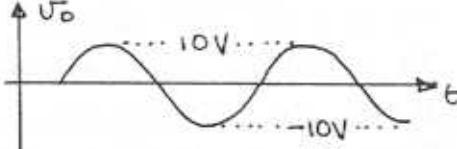
$$V_{p+} = \underline{10V} \quad V_{p-} = \underline{-10V} \quad f = 1\text{kHz}$$
