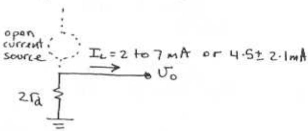
$$\text{Load Regulation} = \frac{\Delta U_o}{I_L} = -2R_d = -\frac{2nVt}{I_D}$$
