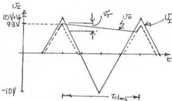
During the diode's off interval, the capacitor discharges through the resistor  $R$  according to :
