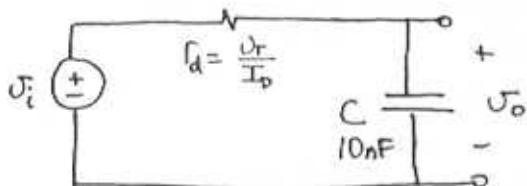
$$\frac{V_o}{V_i} = \frac{\gamma_{sc}}{\gamma_{sc} + r_d} = \frac{1}{1 + sCr_d}$$
