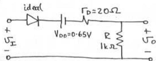
$$U_O = \frac{U_I - V_{D0}}{R + r_D} R, \text{ for } U_I \geq 0.65V$$
