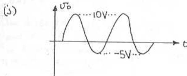
$$V_{p+} = \underline{10V} \quad V_{p-} = \underline{-5V} \quad f = 1kHz$$
