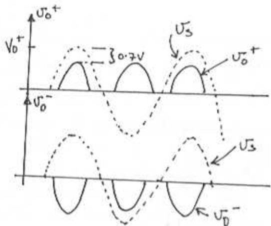
$$\begin{aligned} V_{D,\text{avg}} &= \frac{1}{2\pi} \int V_s \sin \phi - 0.7 \, d\phi = 15 \\ &= \frac{2V_s}{\pi} - 0.7 = 15 \quad \text{assumed } V_s > 0.7V \\ V_s &= \frac{15 + 0.7}{2} \pi = 24.66V \end{aligned}$$
