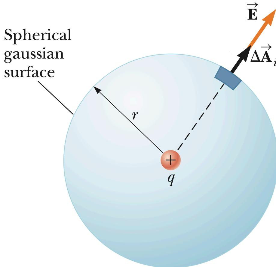
The electric flux through the spherical surface is
