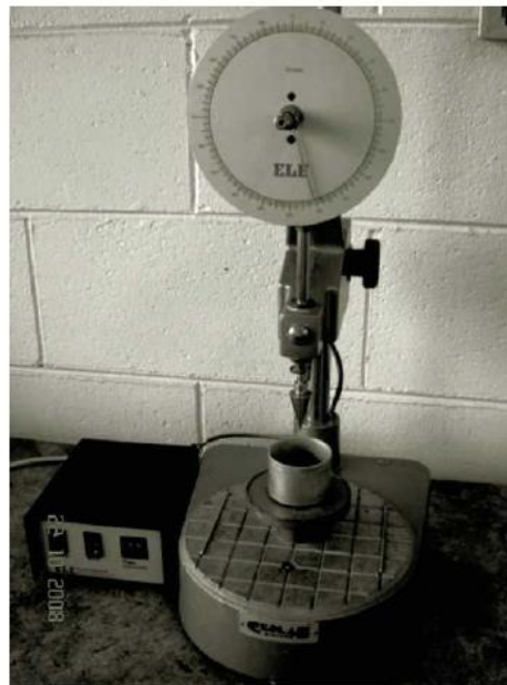
Figure 4.8 Fall cone apparatus (Courtesy of N. Sivakugan, James Cook University, Australia)
