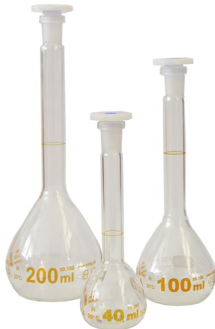
Volumetric flask; contain an accurate volume
