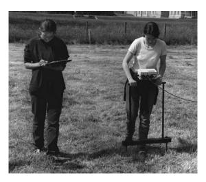
**Figure 1.10** Students using a resistivity meter
