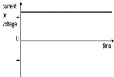
The voltage or current supplied by an DC source are constant with time.
