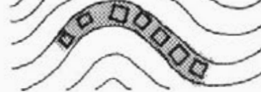
CONFORM BUILDING TO CONTOURS
