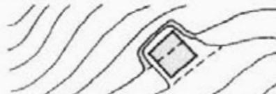
NOTCH FOR BUILDING PLATFORM
