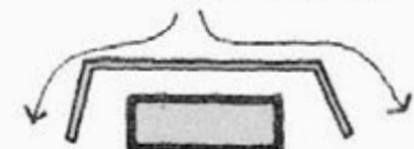
DIVERT DRAINAGE WITH WALL
