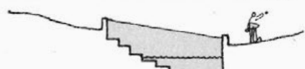
AVOID SUNKEN AREAS THAT CAN'T BE DRAINED
