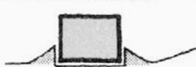
PROTECT BUILDING WITH BERMS
