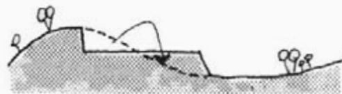
CUT = FILL FOR BUILDING PLATFORM
