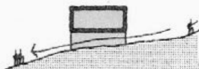
RAISE BUILDING TO ALLOW DRAIN
