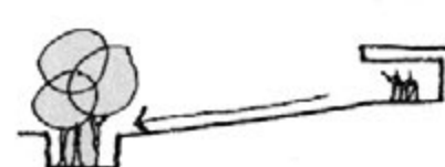
SLOPE EXTERIOR USE AREAS FOR POSITIVE DRAINAGE
