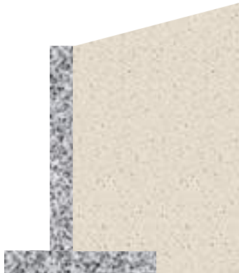
Cantilever retaining wall
