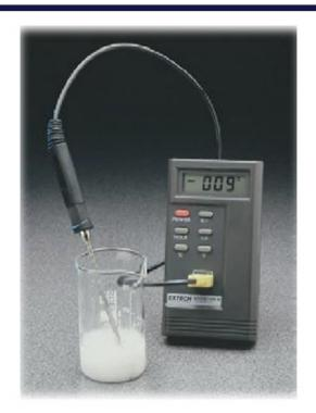
When ammonium thiocyanate and barium hydroxide octahydrate are mixed at room temp., and endothermic reaction occurs:
