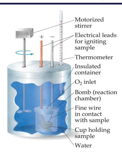
Bomb calorimeter used to measure heat accompanying combustion reactions at constant volume.
