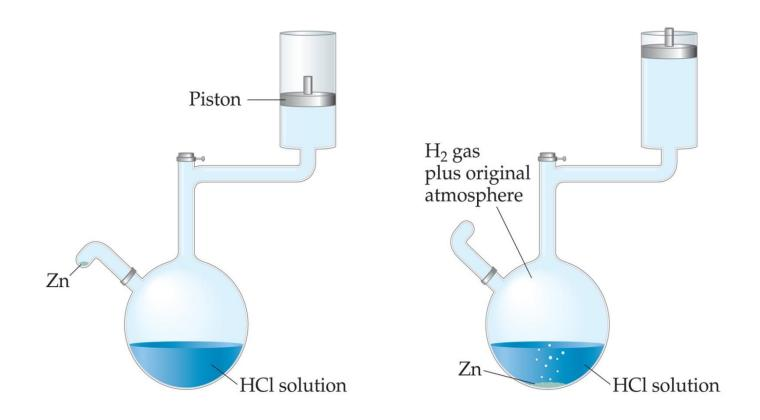
A system that does work on its surroundings. Reaction of zinc metal with HCl at constant pressure. The piston is free to move up and down in its cylinder to maintain a constant pressure equal to atmospheric pressure inside the apparatus. When zinc is added to the acid solution, hydrogen (H<sub>2</sub>) gas is evolved. The H<sub>2</sub> gas does work on the surroundings, raising the piston against atmospheric pressure to maintain constant pressure inside the reaction vessel.
