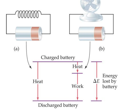
(a) A battery shorted out by a wire (resistance) loses energy to the surroundings only as heat; no work is performed by the system. (b) A battery discharged through a motor loses energy as work (to make the fan turn) with small amount of heat. w and h are different in two cases but E is same.
