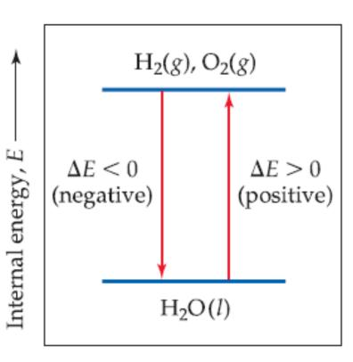
Energy diagram, shows that the internal energy of the  $H_2$  and  $O_2$  mixture is greater than that of  $H_2O$ .
