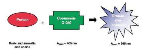
Figure 3. Protein estimation principle using the Bradford method. (9)
