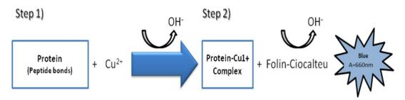
Figure 1. Series of reaction on Lowry method. (5)
