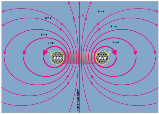
Representing the Coulomb gauge magnetic vector potential **A**, magnetic flux density **B**, and current density **J** fields around a toroidal inductor of circular cross section. Thicker lines indicate field lines of higher average intensity. Circles in the cross section of the core represent the **B**-field coming out of the picture, plus signs represent **B**-field going into the picture.  $\nabla \cdot \mathbf{A} = 0$  has been assumed.
