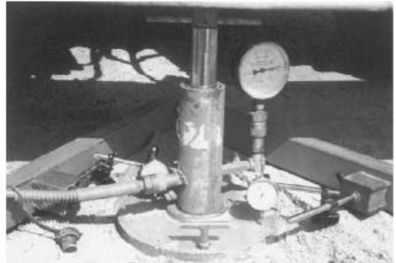
FIGURE 9.36 Plate load test in the field (Courtesy of Braja M. Das, Henderson, Nevada)
