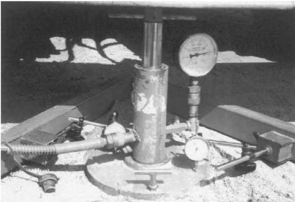
Plate load test in the field
