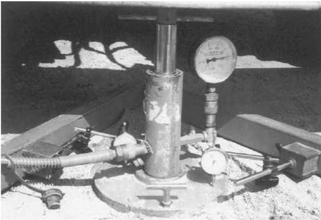
Plate load test in the field
